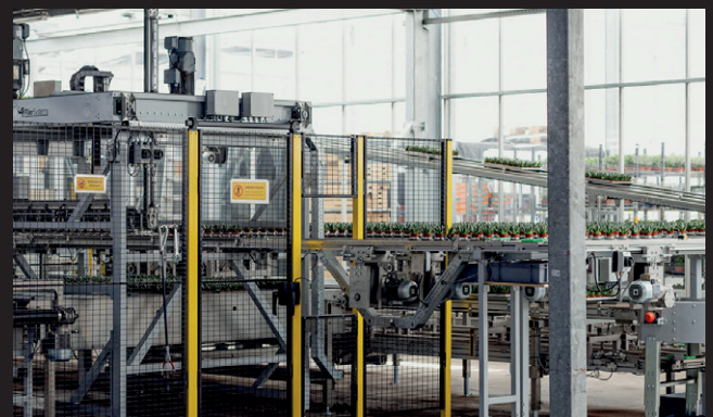
All plants pass through the enormous sorting machine. They are automatically sorted. From that moment, it is known how long it will take before each plant can be delivered.
